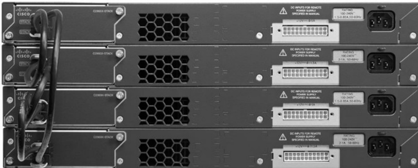
Figure 5. Cisco FlexStack-Plus switch stack
