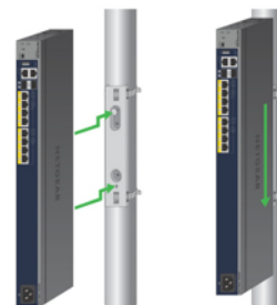
Attaching the Switch to a Round Pole
