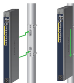
Attaching the Switch to a Round Pole
