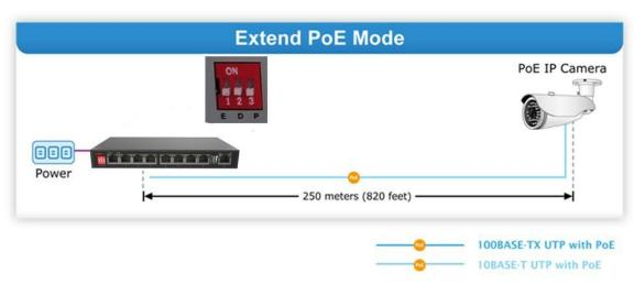
Extend network communication distance and PoE power supply distance.
